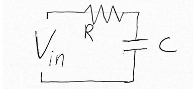
**TLDR:** We can use these simple laws, along with Kirchhoff's loop rule (the total voltage around any circle must always be zero) to see that the simple RC circuit above must obey the ODE:
